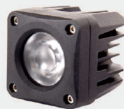
JC1001-10W LED Power: 10W Raw Lumens: 860 LM Current: 1.01A@12V
